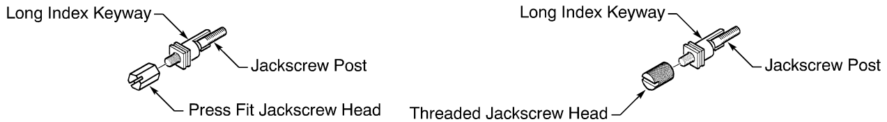
OBsolete JACKSCREW ASSEMBLY Figure 3
